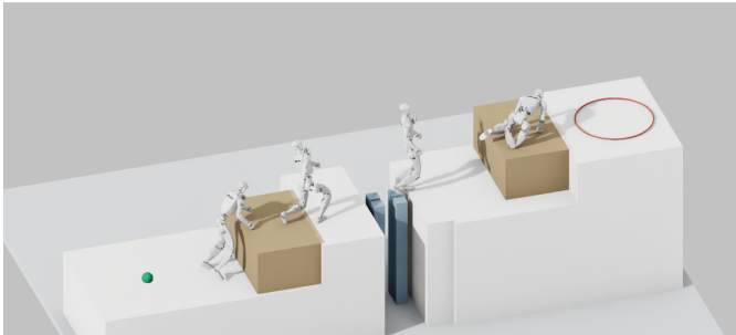
Fig. S1. Eight curated composite courses used for evaluation. Each panel shows four successive robot poses from one successful traversal. Green markers indicate starting positions, and red circles show the 0.5 m horizontal goal tolerance. Success rates for Ours and MGMT are measured over 1,000 episodes per method and course.
